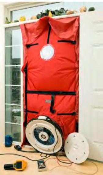
House undergoing a blower door test. Test provides a measured air leakage rate and can help identify areas in the building envelope that need to be addressed to improve airtightness.
